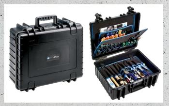
internal dimensions  $473 \times 351 \times 197 \text{ mm}$  | payload 30 kg | weight 6.4 kg | material PP description airworthy, strong, dustproof, waterproof, document pocket in the lid, 2 removable tool boards, variable bottom tray with aluminum divider system
